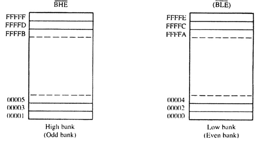
Note:  $A_0$  is labeled  $\overline{BLE}$  (Bus low enable) on the 80386SX.
